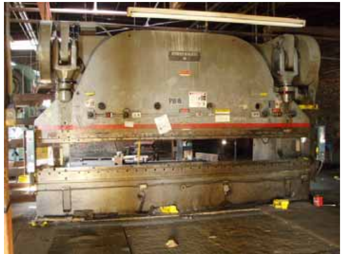
Press Brake, Cincinnati 13, s/n 37054, 12', 400 ton
