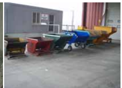
Dump Hoppers - Partial View
